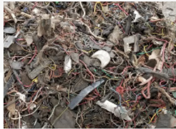
SHREDDER WIRES / ASR
